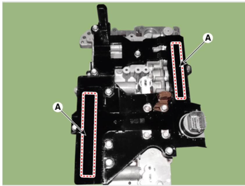
7. Remove the solenoid valve support bracket (A).
